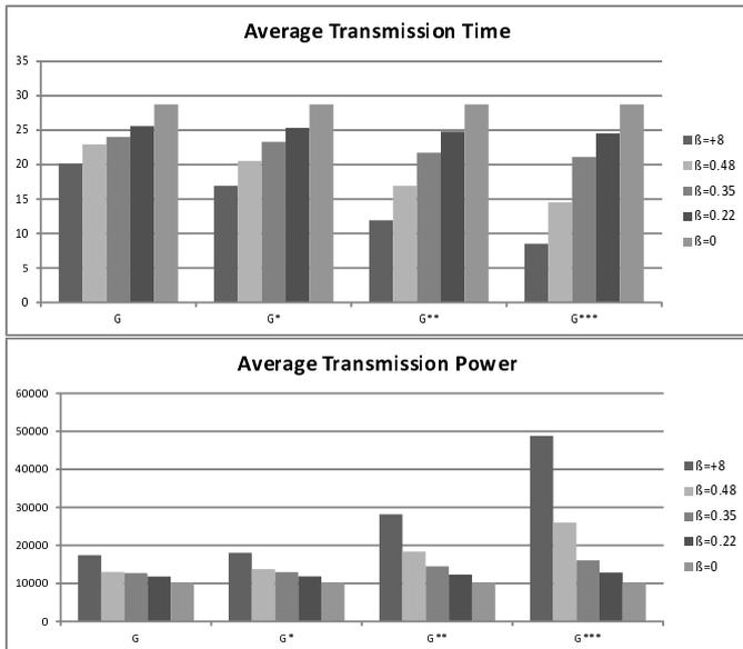
Fig. 9 Average transmission time and power in Experiment 2
